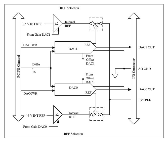
Figure 3-9. Analog Output Circuitry Block Diagram
