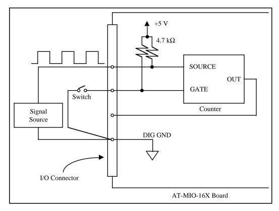
Figure 2-17. Event-Counting Application with External Switch Gating
