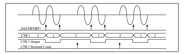
Figure 3-15. FIFO Pulsed Waveform Generation Timing
