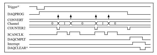
Figure 3-8. Interval Scanning Posttrigger Data Acquisition Timing
