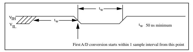
Figure 2-15. EXTTRIG\* Signal Timing
