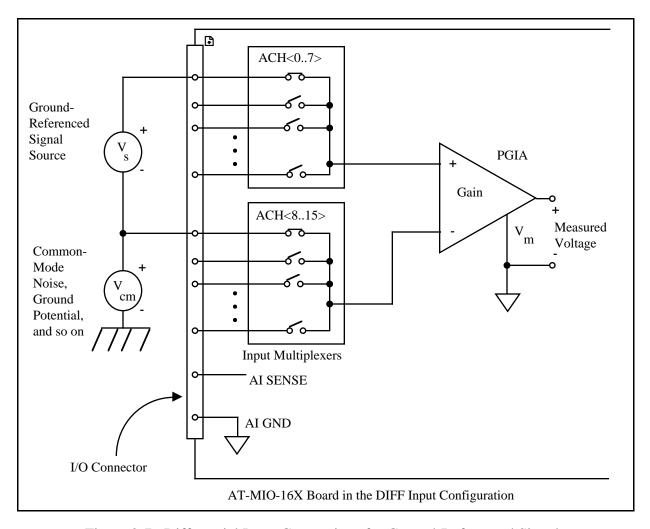
Figure 2-7. Differential Input Connections for Ground-Referenced Signals
