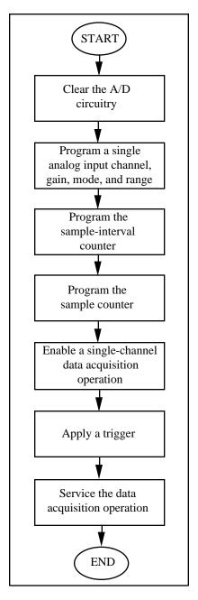
Figure 5-3. Single-Channel Data Acquisition Programming
