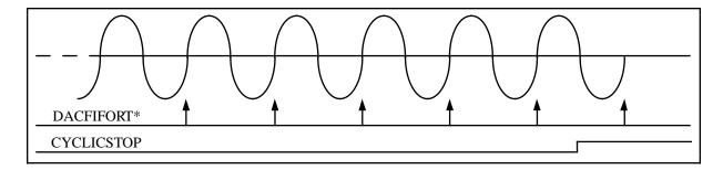
Figure 3-13. FIFO Cyclic Waveform Generation with Disable
