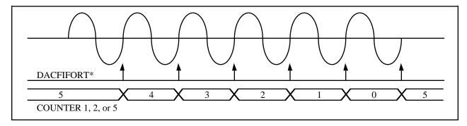
Figure 3-14. FIFO Programmed Cyclic Waveform Timing
