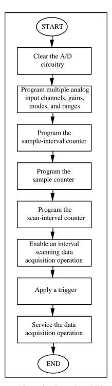
Figure 5-5. Interval Scanning Data Acquisition Programming
