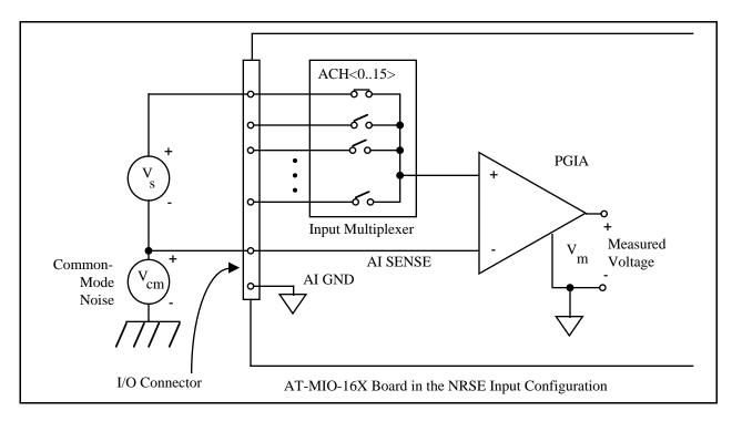
Figure 2-10. Single-Ended Input Connections for Ground-Referenced Signals
