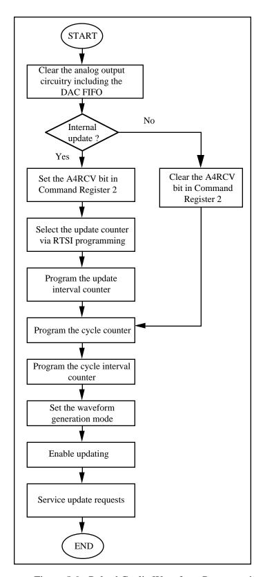
Figure 5-9. Pulsed Cyclic Waveform Programming
