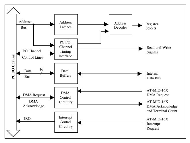
Figure 3-2. PC I/O Channel Interface Circuitry Block Diagram
