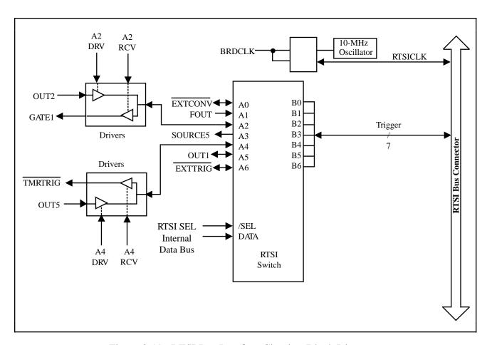
Figure 3-19. RTSI Bus Interface Circuitry Block Diagram
