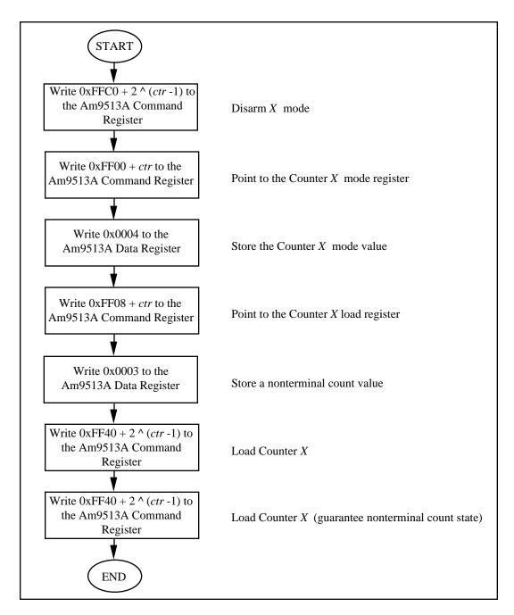
Figure 5-6. Resetting an Am9513A Counter/Timer
