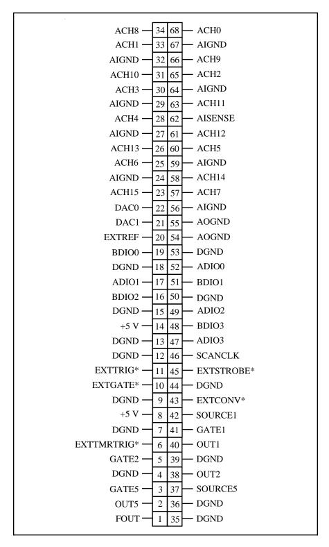
Figure B-2. AT-MIO-16X 68-Pin I/O Connector
