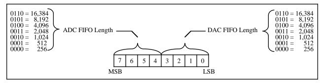
Figure 6-4. ADC and DAC FIFO Depth Field
