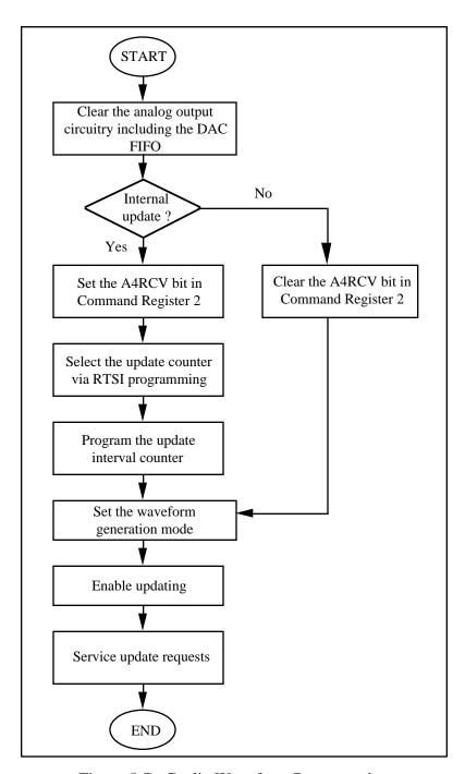
Figure 5-7. Cyclic Waveform Programming
