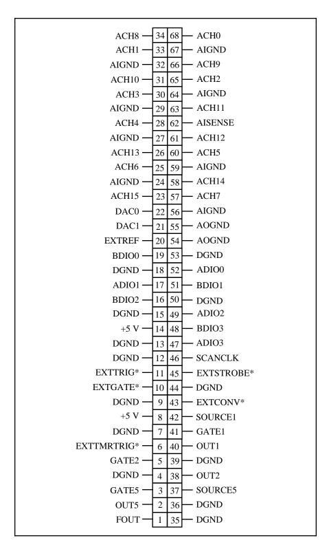
Figure 2-5. AT-MIO-16X 68-Pin I/O Connector
