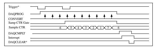
Figure 3-6. Single-Channel Pretrigger Data Acquisition Timing
