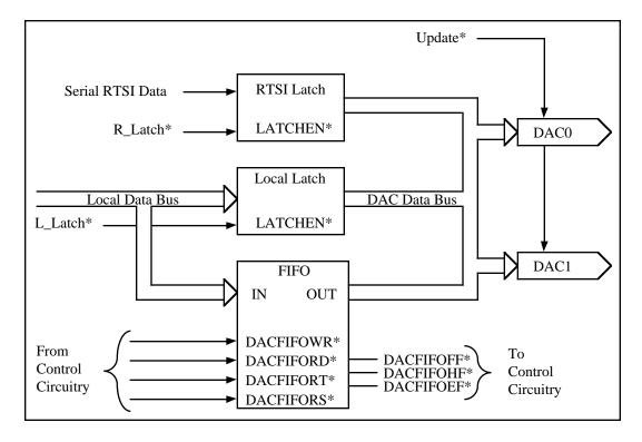
Figure 3-10. Analog Output Waveform Circuitry
