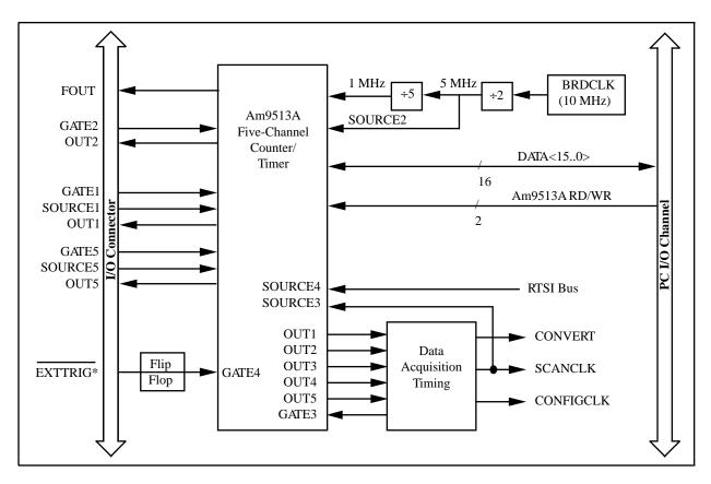
Figure 3-17. Timing I/O Circuitry Block Diagram
