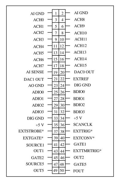
Figure B-1. AT-MIO-16X 50-Pin I/O Connector
