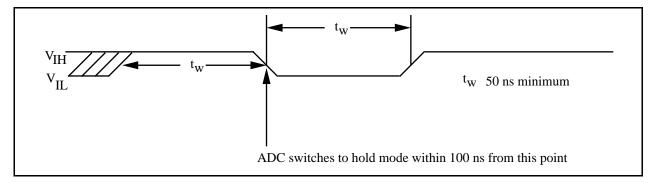
Figure 2-14. EXTCONV\* Signal Timing
