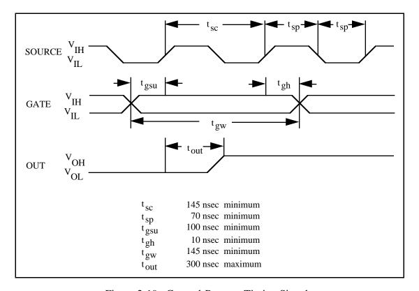
Figure 2-19. General-Purpose Timing Signals
