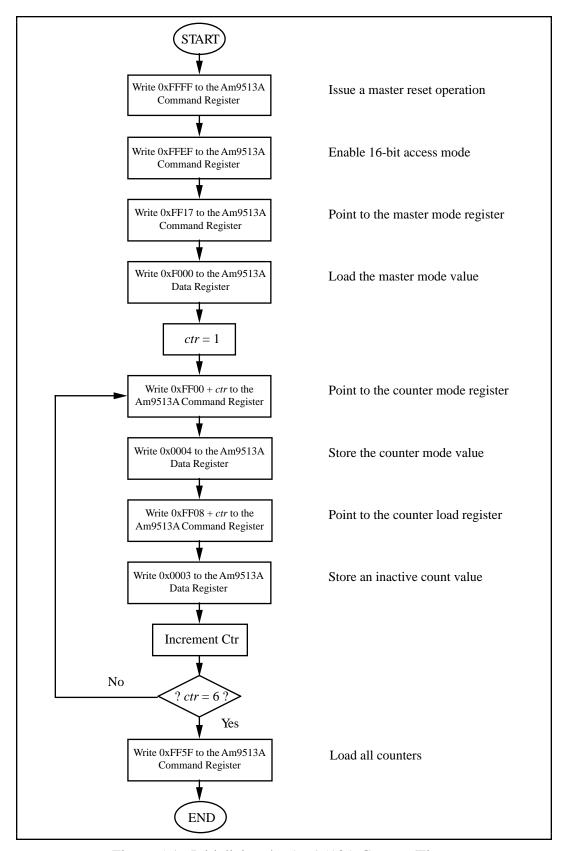
Figure 5-1. Initializing the Am9513A Counter/Timer
