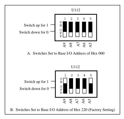
Figure 2-3. Example Base I/O Address Switch Settings
