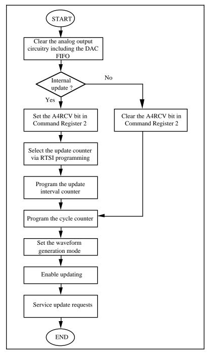
Figure 5-8. Programmed Cycle Waveform Programming
