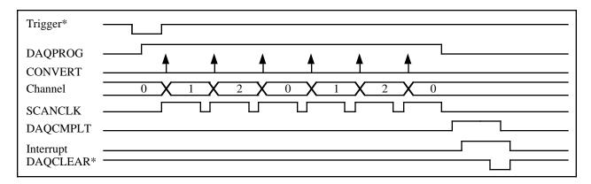
Figure 3-7. Scanning Posttrigger Data Acquisition Timing
