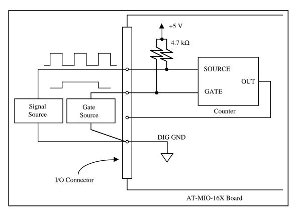
Figure 2-18. Frequency Measurement Application
