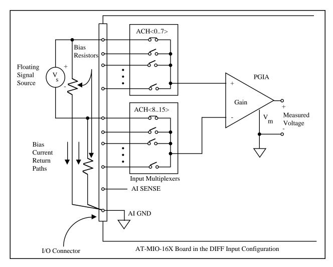
Figure 2-8. Differential Input Connections for Nonreferenced Signals
