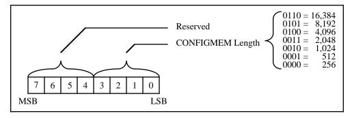
Figure 6-3. Configuration Memory Depth Field
