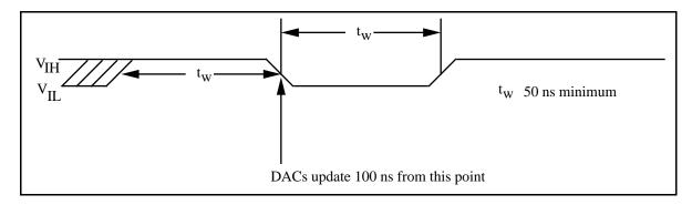
Figure 2-16. EXTTMRTRIG\* Signal Timing
