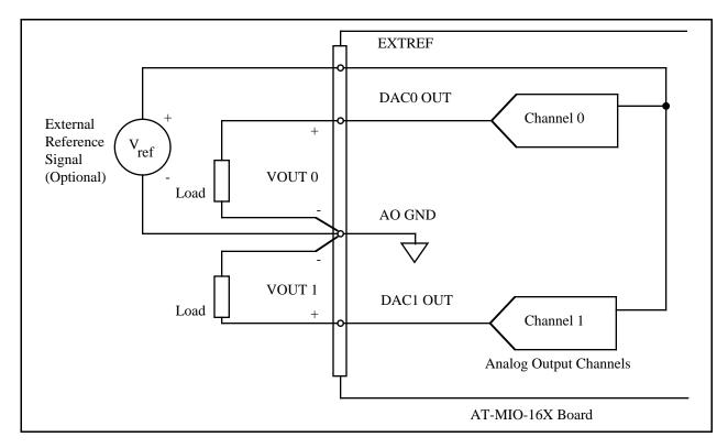
Figure 2-11. Analog Output Connections
