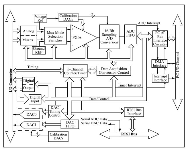
Figure 3-1. AT-MIO-16X Block Diagram
