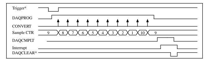
Figure 3-5. Single-Channel Posttrigger Data Acquisition Timing
