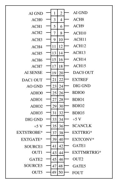
Figure 2-4. AT-MIO-16X 50-Pin I/O Connector
