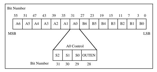
Figure 5-10. RTSI Switch Control Pattern
